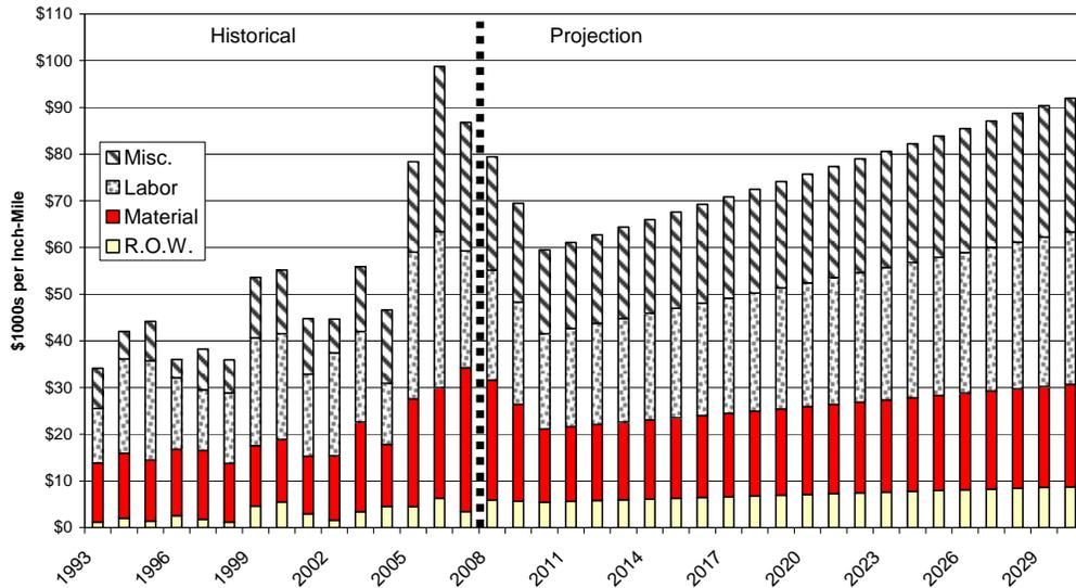
*Average of large-diameter gas pipelines 30 to 36 inches FERC data compiled by Oil & Gas Journal 2010 to 2030 projections by cost component is based on trends from 1993 to 2004. Miscellaneous includes surveys, engineering, supervision, interest, administration, overheads, contingencies, allowances for funds used during construction (AFUDC) and FERC fees.*
