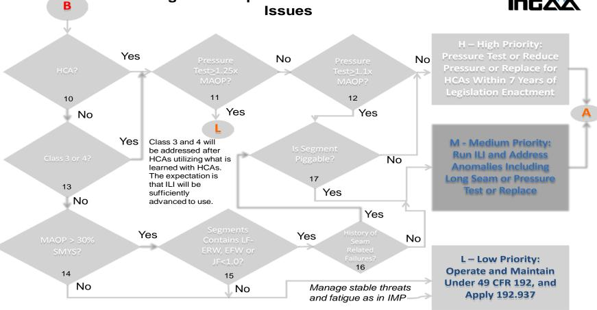
LF-ERW is low frequency electric resistance welded; EFW is electric fusion or flash welded; and JF is joint factor as defined at 49 CFR 192.113
