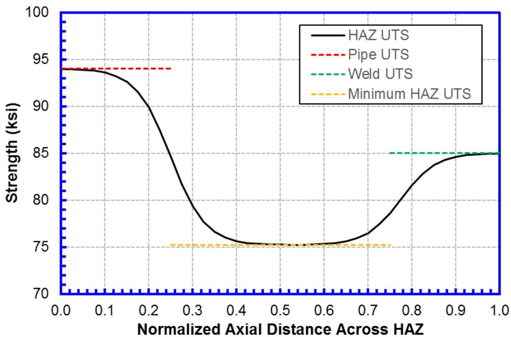
Figure 24. Schematic of HAZ Strength
