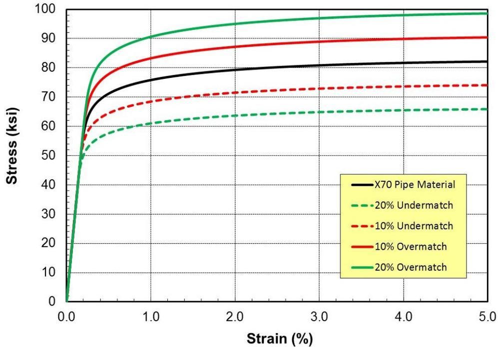
**Figure 1. Schematic Stress-Strain Curves Showing Weld Metal Under-Matching and Over-Matching**
