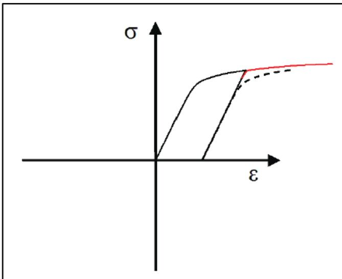
**Figure 4. Strain Hardening**
