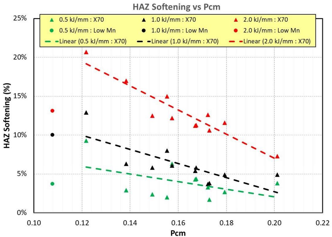
Figure 14. HAZ Softening (%) vs. Carbon (%) and Pcm
