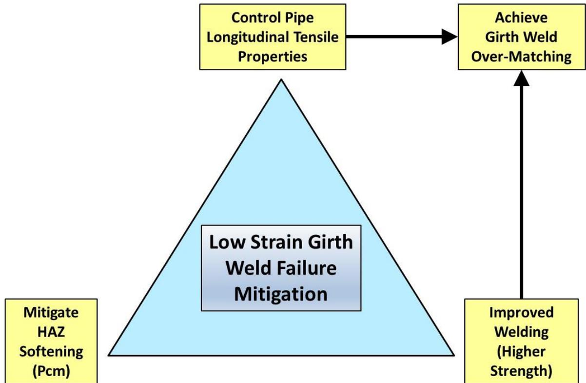
Figure 26. Low Strain Girth Weld Failure Mitigation Strategy
