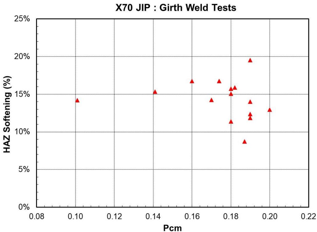
Figure 19. Average HAZ Softening (%) as a Function of Carbon (%) and Pcm
