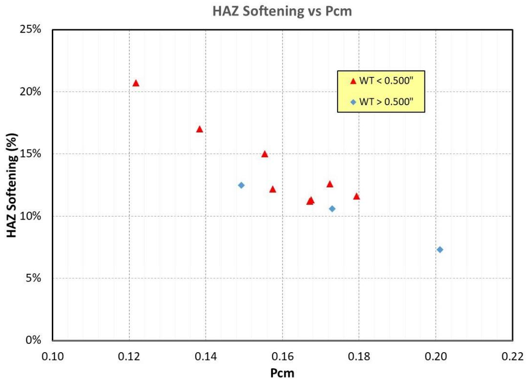
Figure 15. HAZ Softening (%) vs. Pcm
