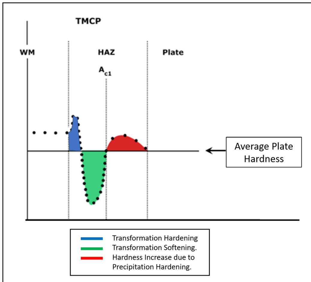
Figure 8. Schematic of Hardness Variation across the Heat Affected Zone
