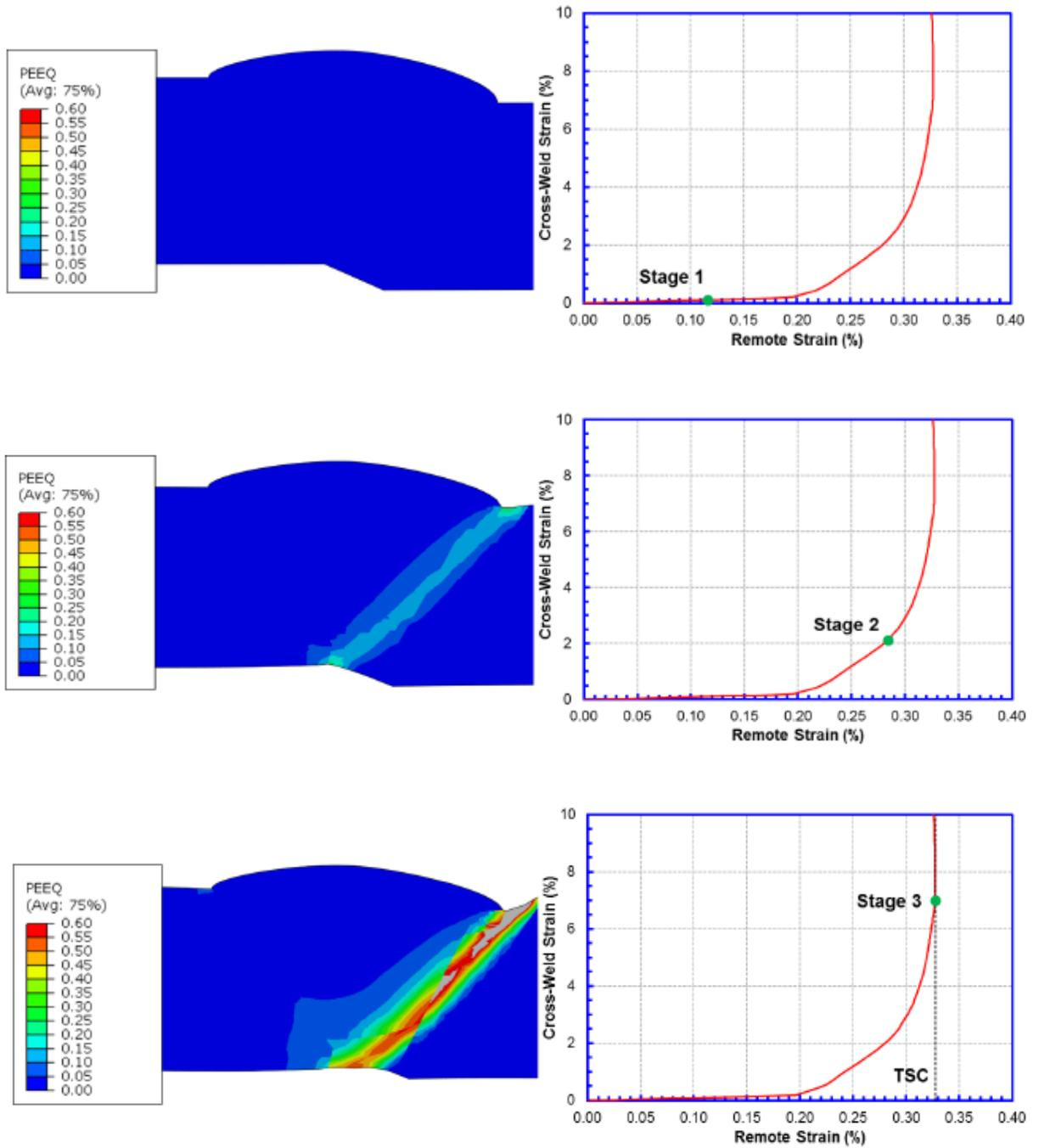
Figure 25. Development of Strain in an Under-matched Girth Weld
