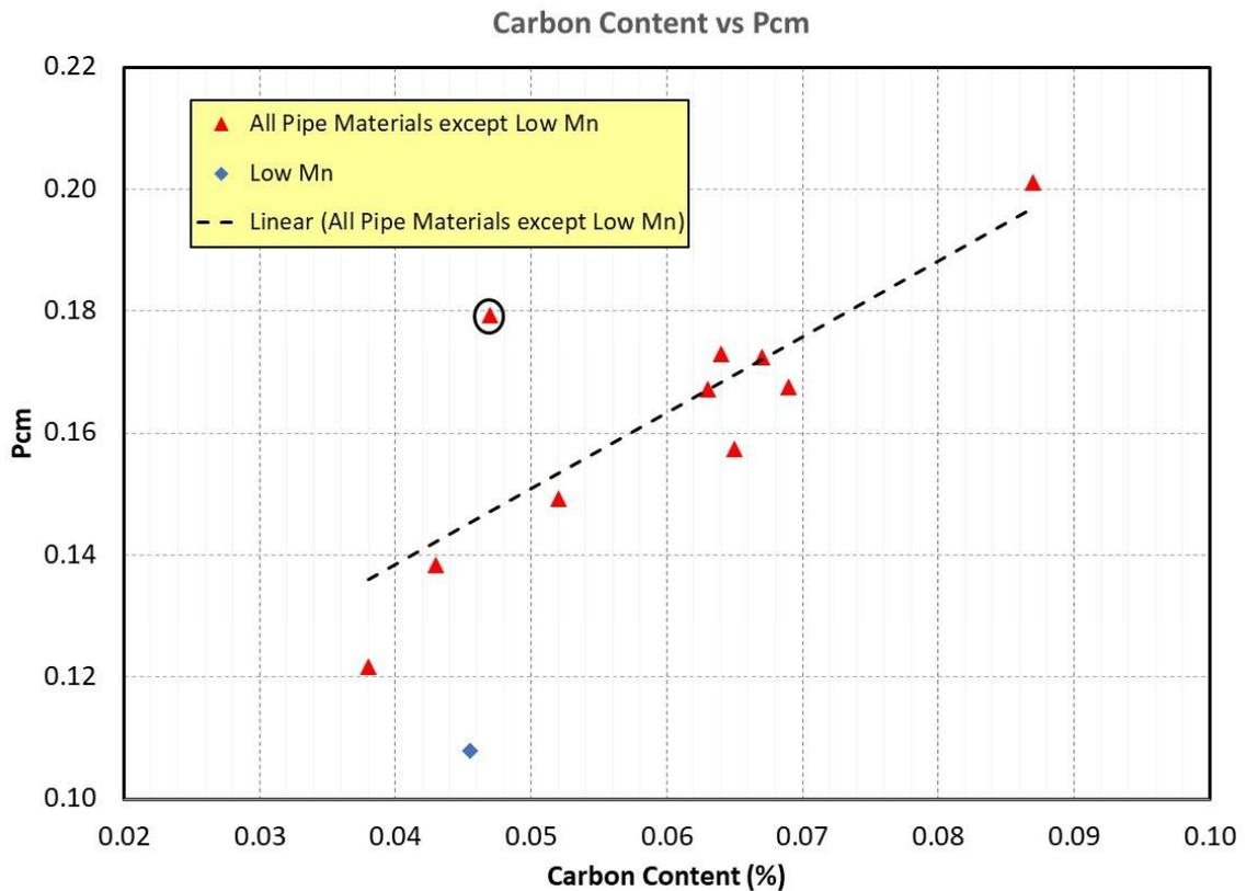
**Figure 10. Plot of Carbon Content (%) vs. Pcm for BOP Pipe Materials**
