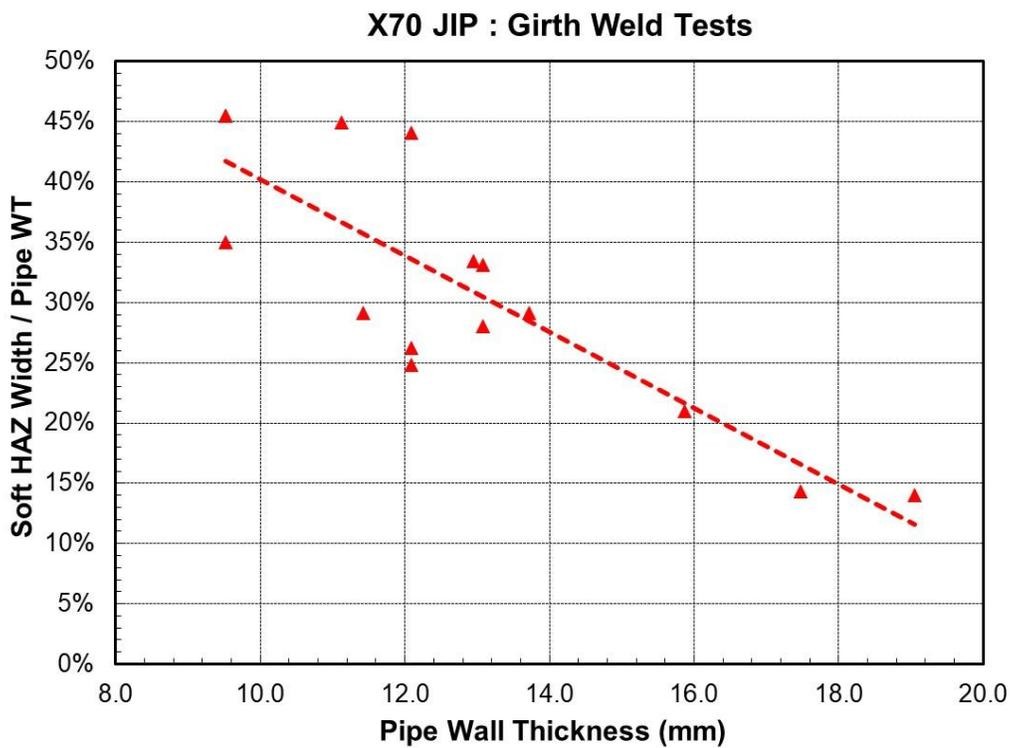
Figure 21. Width of Softened HAZ Softened Zone vs. Pipe Wall Thickness
