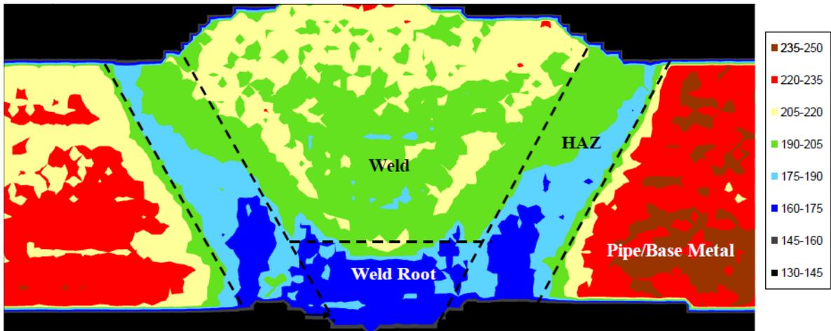
**Figure 2. Hardness Map of a Girth Weld in Incident 1**
