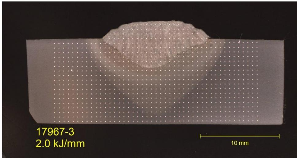
**Figure 11. Typical Macro after Microhardness Testing (2.0 kJ/mm)**
