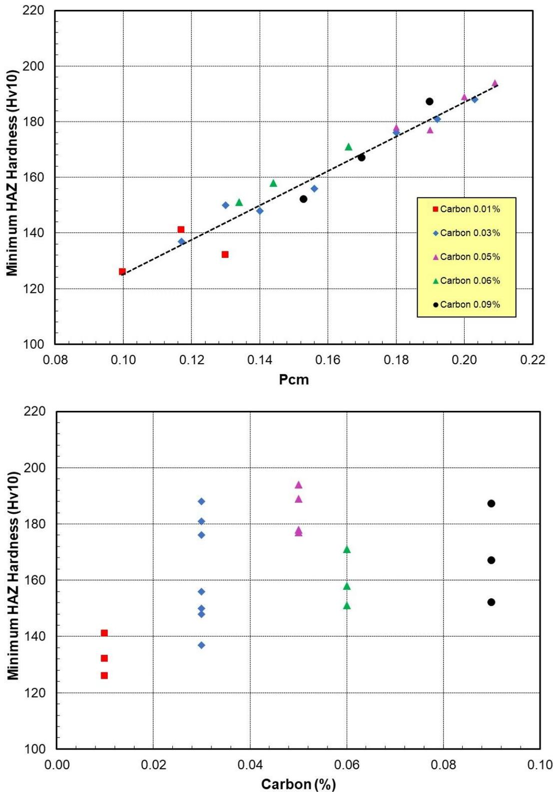
Figure 9. Plots of Minimum HAZ Hardness vs. Carbon (%) and Pcm
