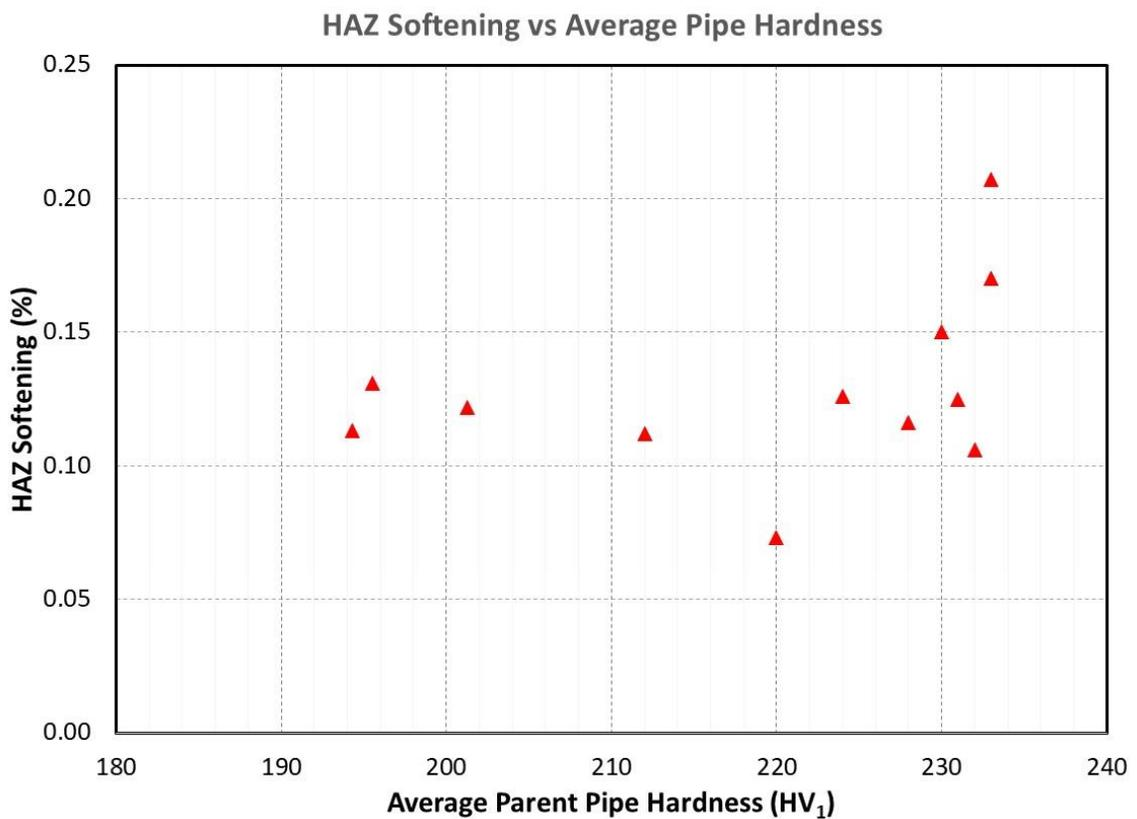
Figure 16. HAZ Softening (%) vs. Average Pipe Hardness
