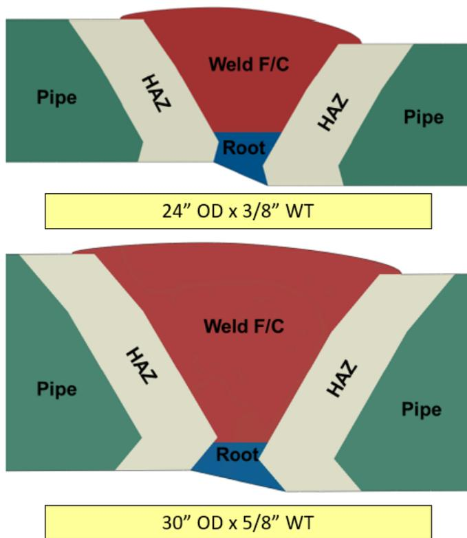
Figure 23. Schematic of FEA Models (Regular Weld Cap)
