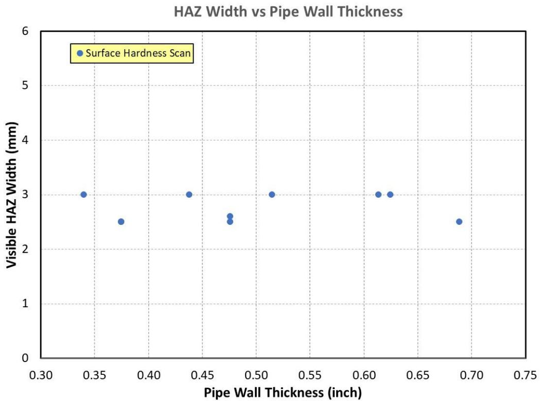
Figure 13. Comparison of Bead on Pipe HAZ Widths vs Pipe WT (2.0 kJ/mm)
