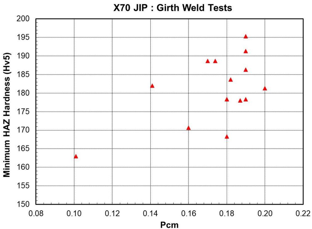
Figure 20. Minimum HAZ Hardness as a Function of Carbon (%) and Pcm
