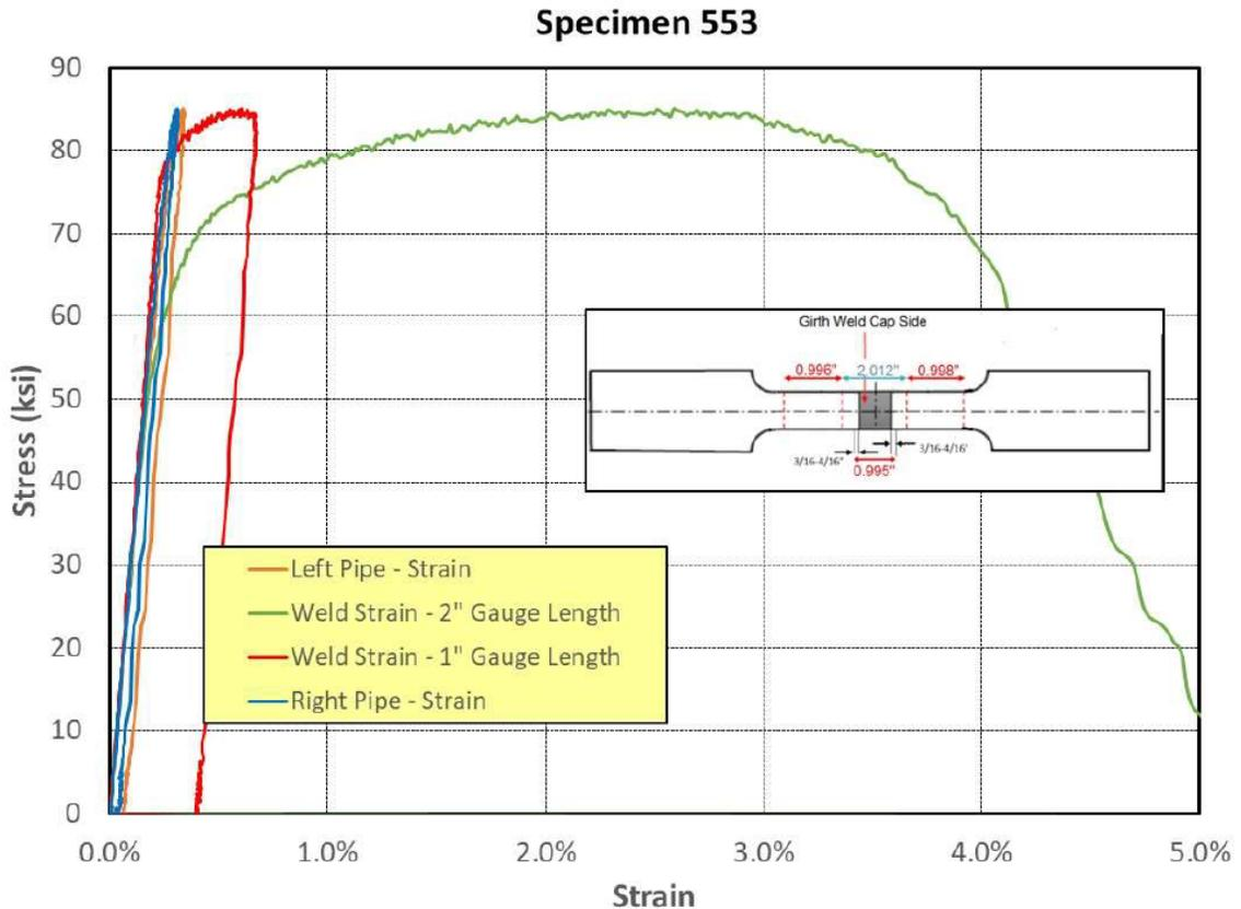
Figure 22. Stress-Strain Plots for Girth Weld 104629 (48" x 0.689")
