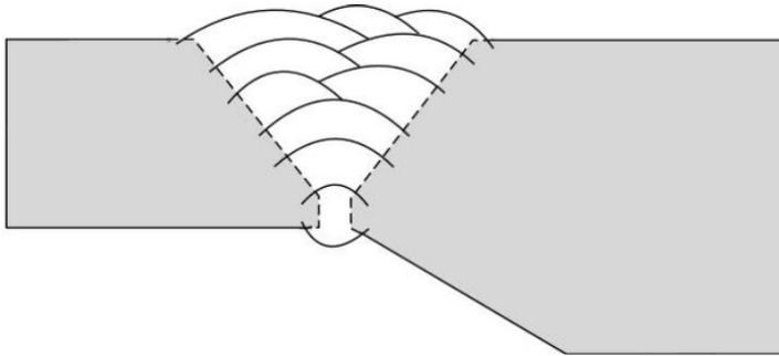
**Figure 7. Schematic Showing Transition Weld with Taper at Pipe End**
