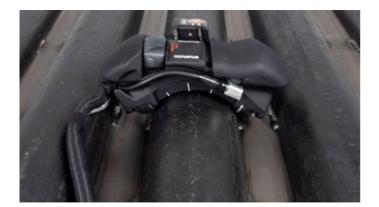
Can also be used for longitudinal scanning on sections of pipe that may not be accessible with an AUT C-Scan unit.
