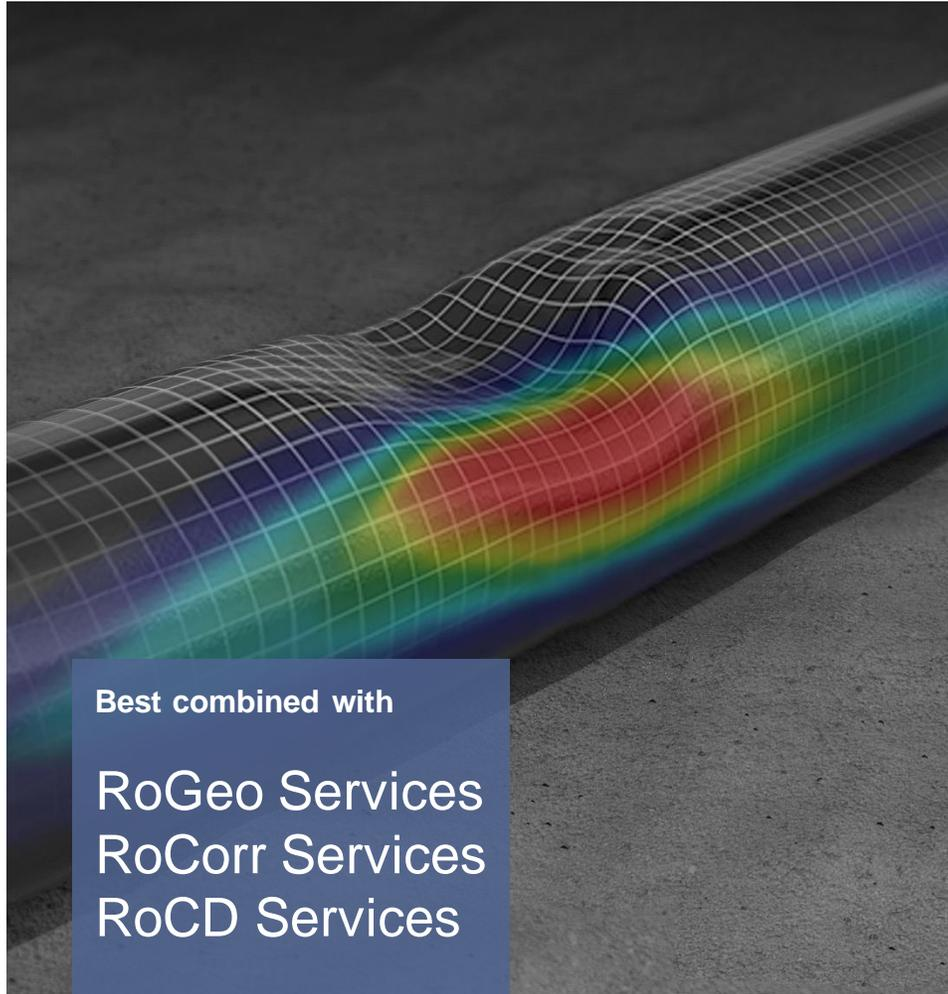
Deformations in pipelines cause stress concentrations and may initiate failure by fatigue. These pose a major threat to pipeline integrity.
