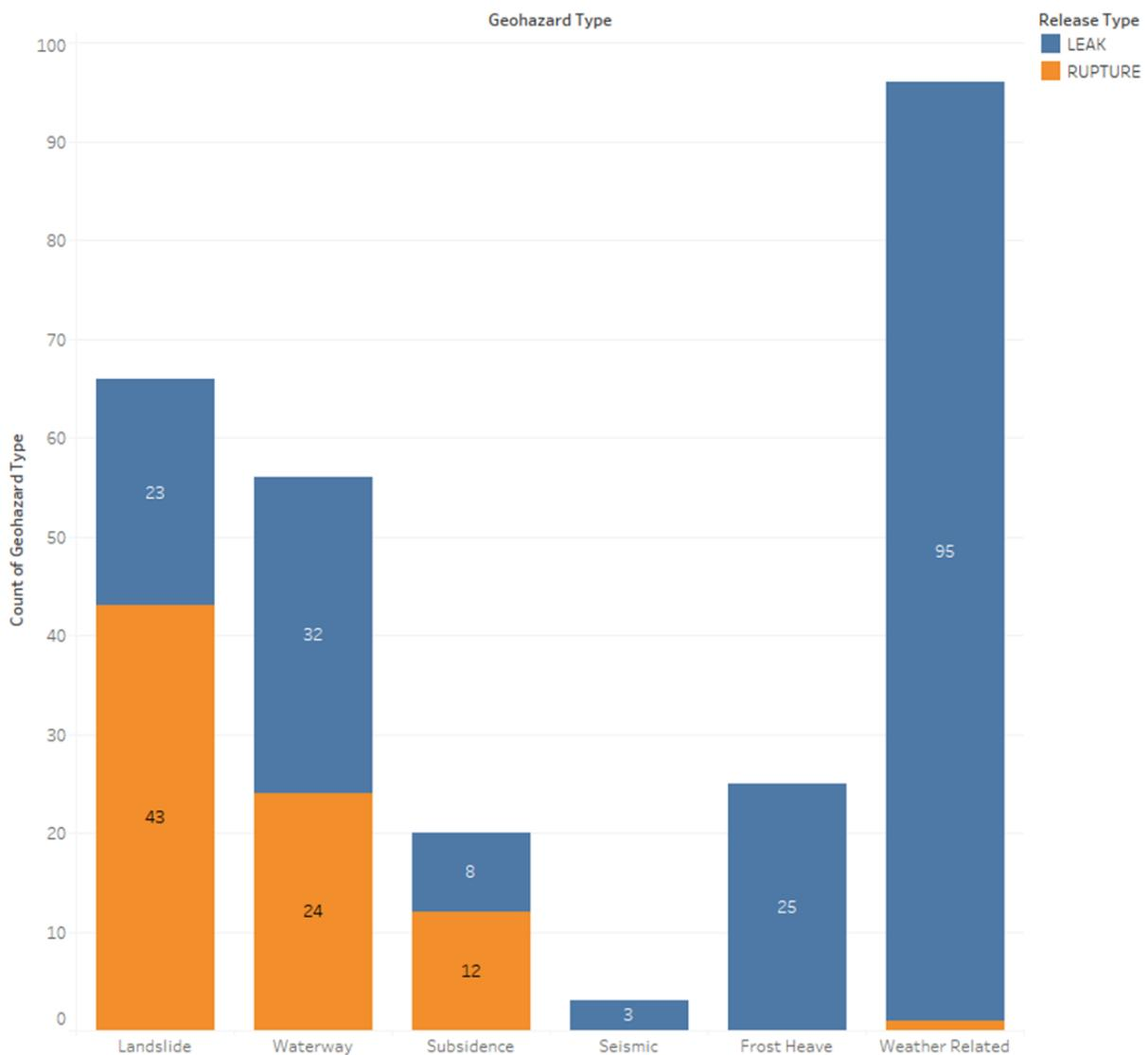
Figure A-1 Incidents by hazards type and leak vs. rupture (over a 20.5-year period)
