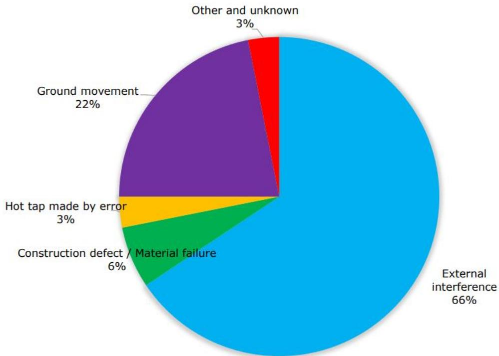
Figure A-14 EGIG distribution of incidents with hole leak size from 2010-2019 [2]
