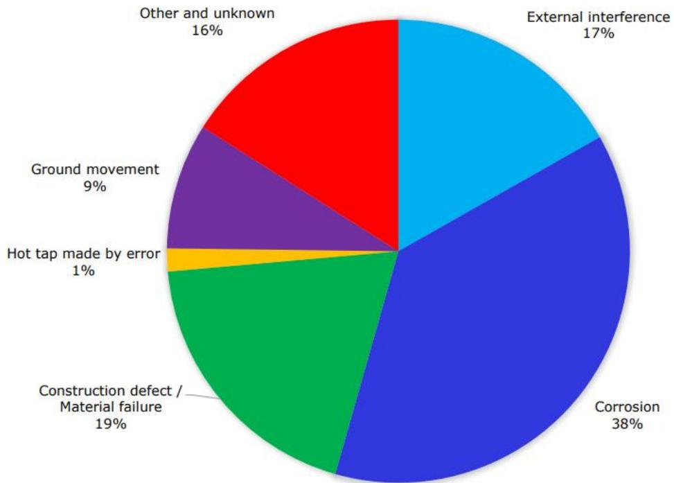
Figure A-13 EGIG distribution of incidents with pinhole/crack leak size from 2010-2019 [2]
