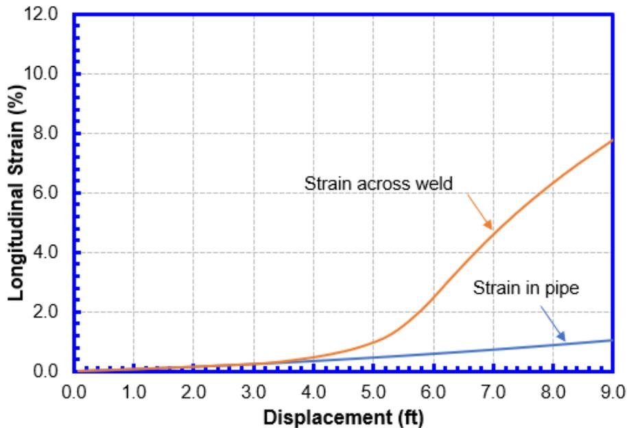
Figure E-6 Comparison of strain across a girth weld and strain in the pipe body in a weld joint with weld strength undermatching
