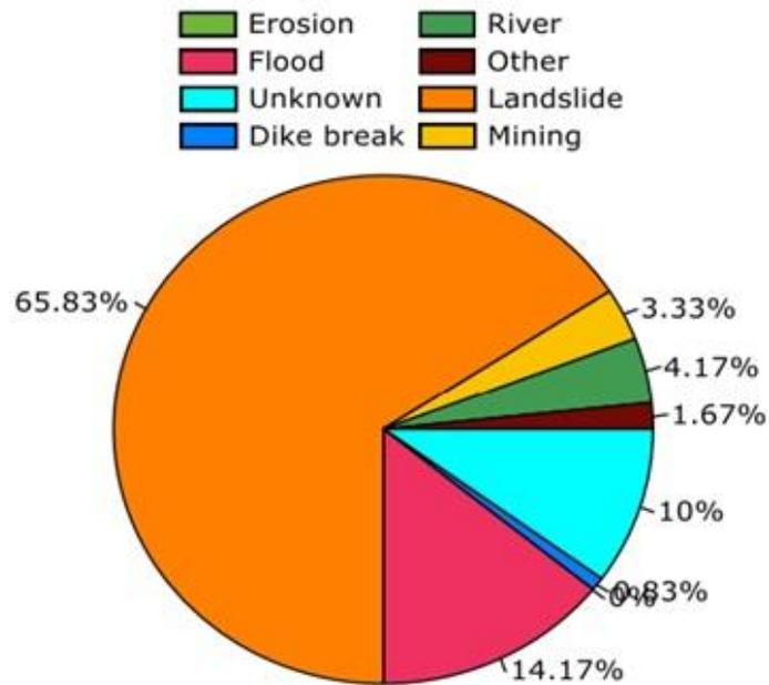
Figure A-18 EGIG distribution of sub-causes of ground movement incidents (period 1970-2019) [2]
