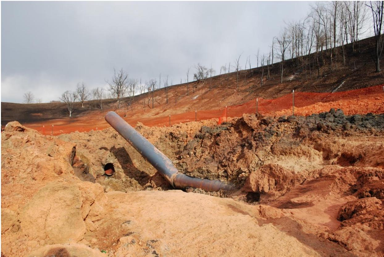
Figure E-2 Failure of a girth weld of a vintage pipeline at low strain due to weld flaws
