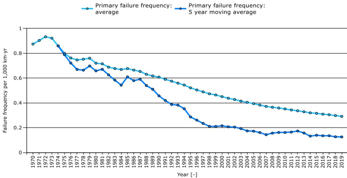
Figure A-11 EGIG primary failure frequency [2]
