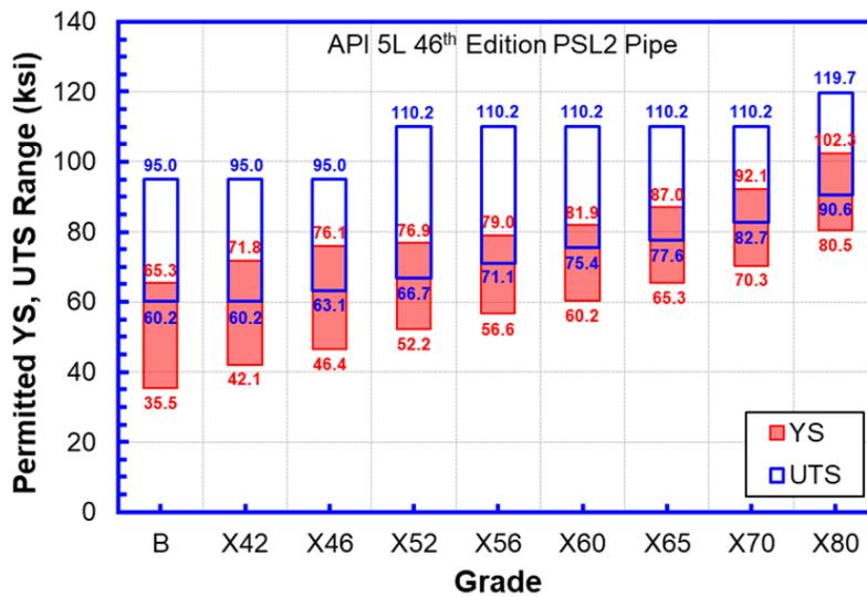
Figure D-2 Permitted ranges of yield strength and UTS for PSL2 pipes in API 5L
