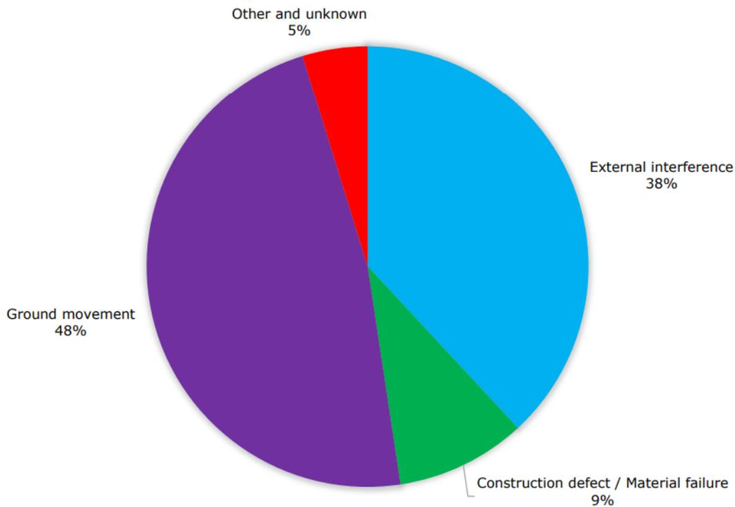
Figure A-15 EGIG distribution of incidents with rupture leak size from 2010-2019 [2]
