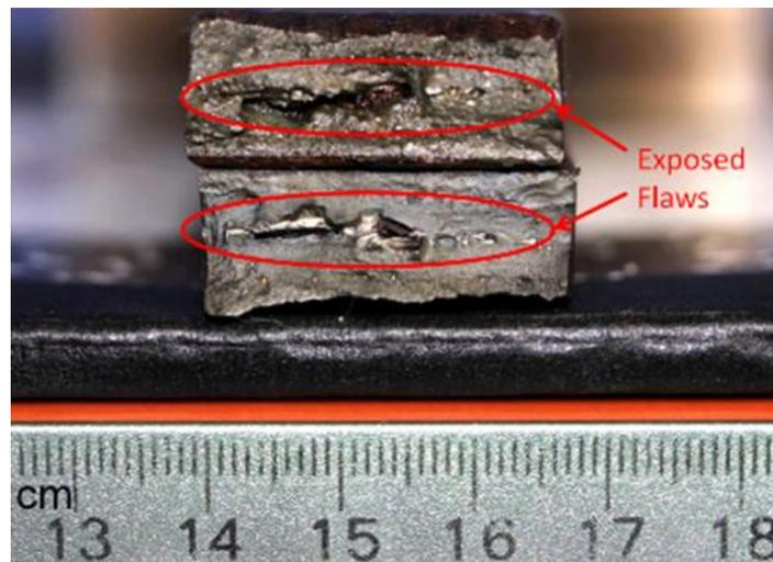
Figure E-1 Exposed flaws at the fracture surface of a girth weld after a cross-weld tensile test
