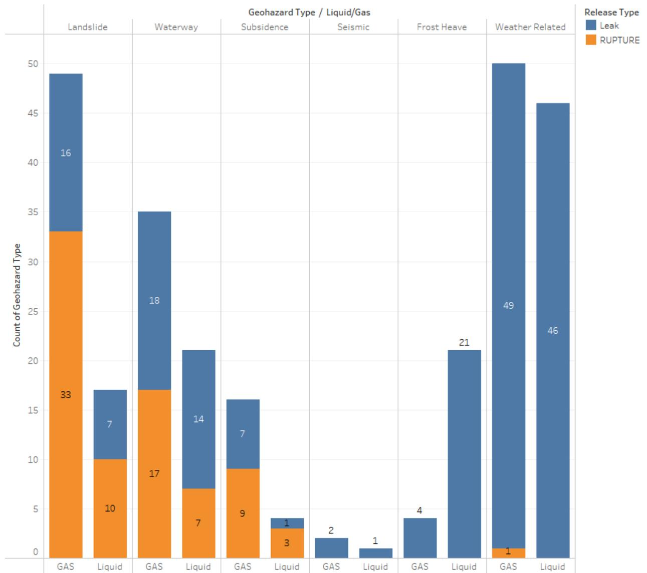
Figure A-2 Incidents by types of pipeline and hazards (over a 20.5-year period)
