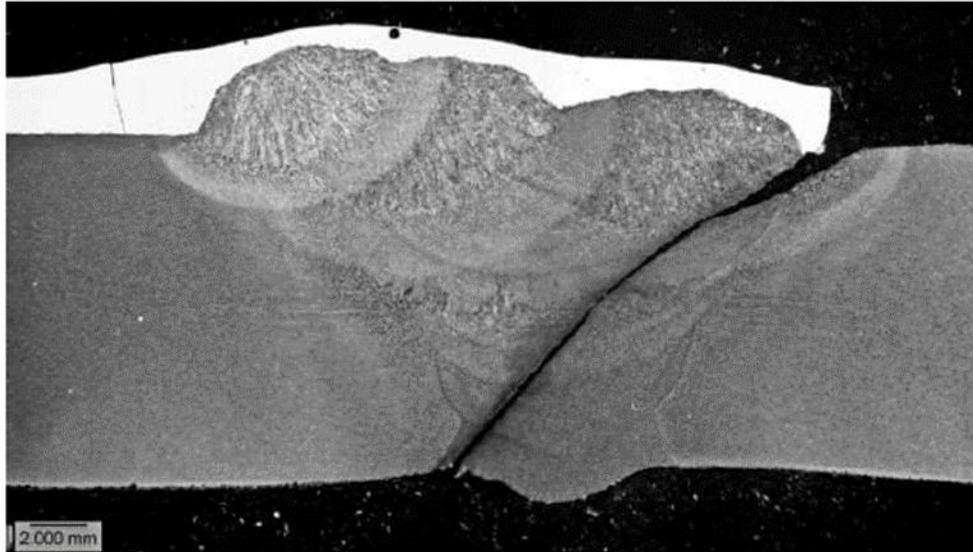
Figure D-1 Example of a failed girth weld with weld strength undermatching
