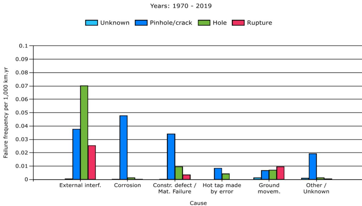
Figure A-16 EGIG primary failure frequency, cause, and size from 1970-2019 [2]
