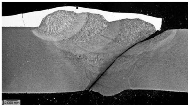
Figure E-4 Failure of a girth weld with weld strength undermatching in the absence of weld flaws
