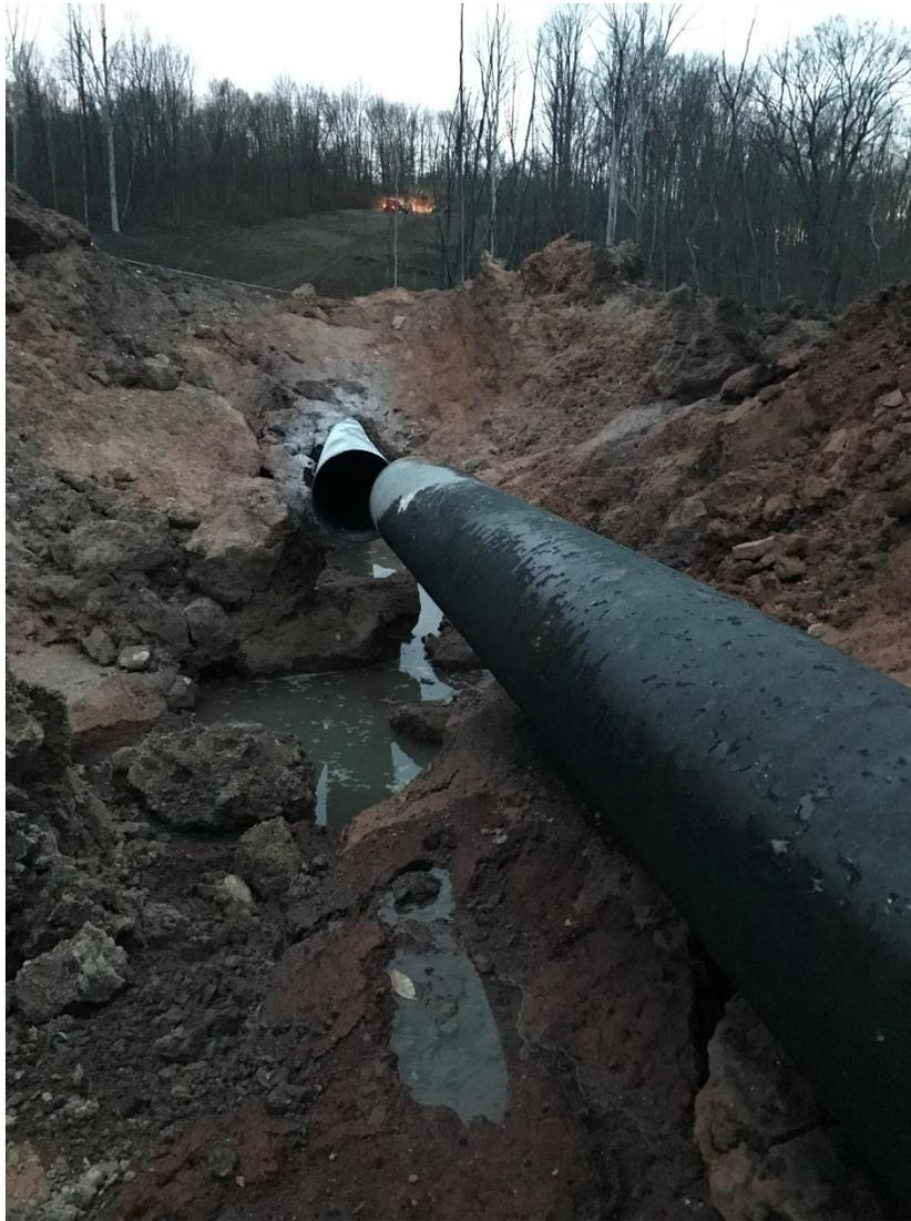
Figure E-5 In-service failure of a girth weld with weld strength undermatching
