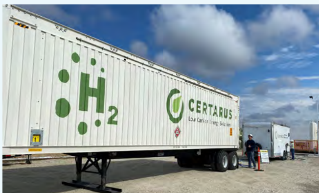
Above: A trailer mounted hydrogen fuel blending system stationed at Southern Star's facility where hydrogen fuel blends were used in GMV engines at a rate up to 30%.
